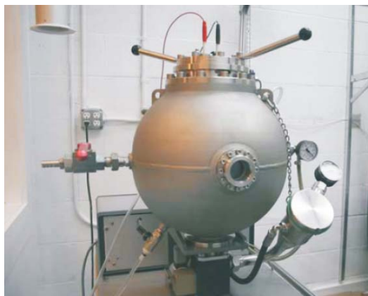
Fig. 2 20-L-Apparatus for determining flammability characteristics of toluene and methanol mixtures [27]
